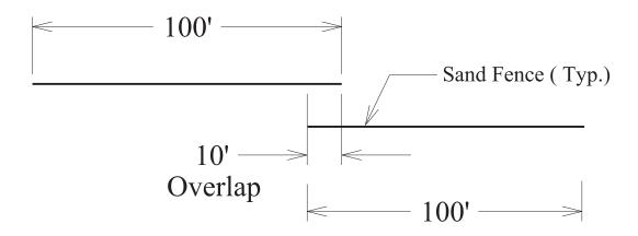
Typical Section #1 will be placed parallel to the roadway, on or near the top of sand dunes as directed by the Engineer
